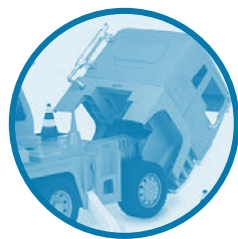
Tilting cab La cabine bascule
