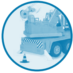
Folding support legs Système de support pliant
